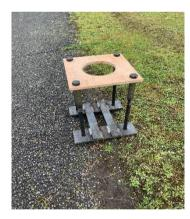
Some passively safe products require an anchor cradle to be embedded into the foundation to support the finished structure. Anchor cradles are suspended into the excavation often by means of wooden batons prior to concrete pour.
